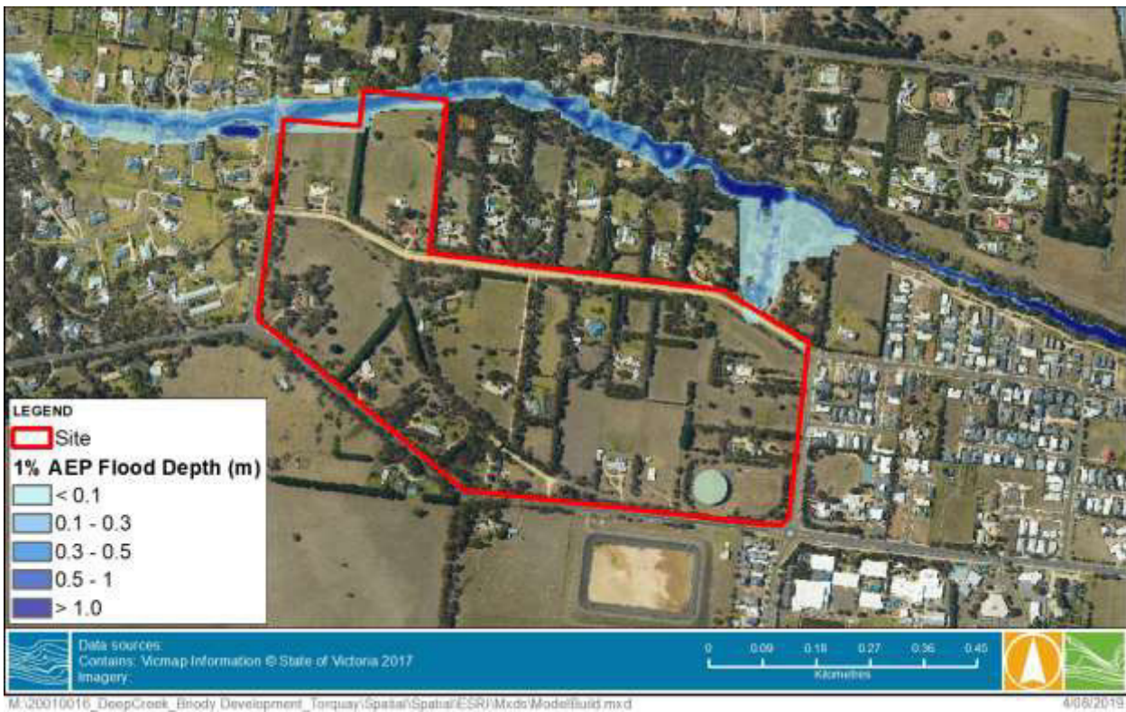
FIGURE 3-4 DEEP CREEK 1% AEP FLOOD DEPTH
