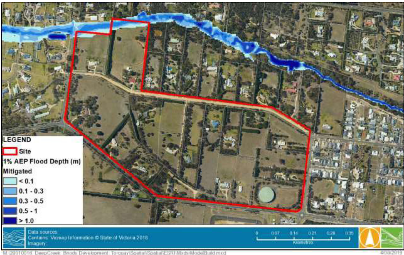
FIGURE 4-7 1% AEP FLOOD DEPTH – MITIGATED CONDITIONS
