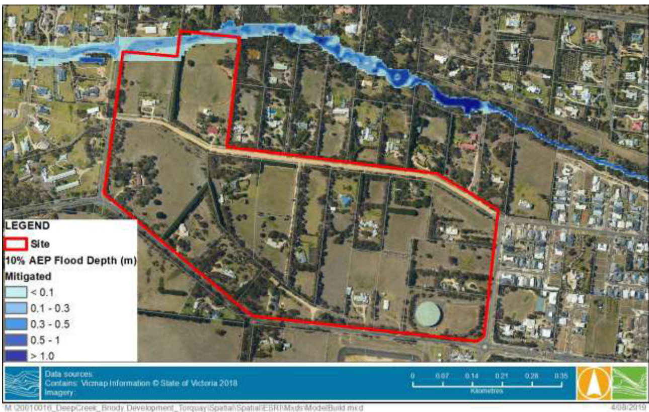
FIGURE 4-8 10% AEP FLOOD DEPTH – MITIGATED CONDITIONS
