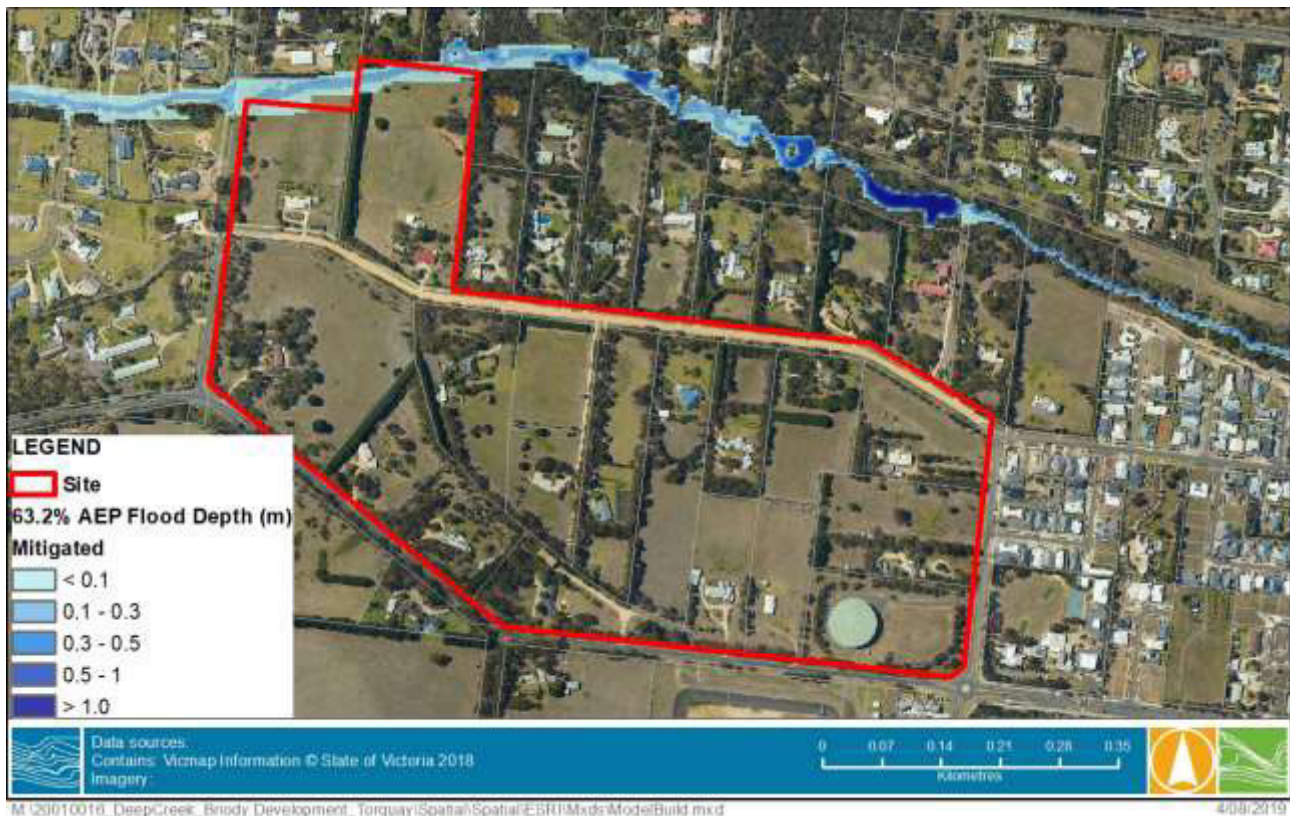
FIGURE 4-9 63.2% AEP FLOOD DEPTH – MITIGATED CONDITIONS
