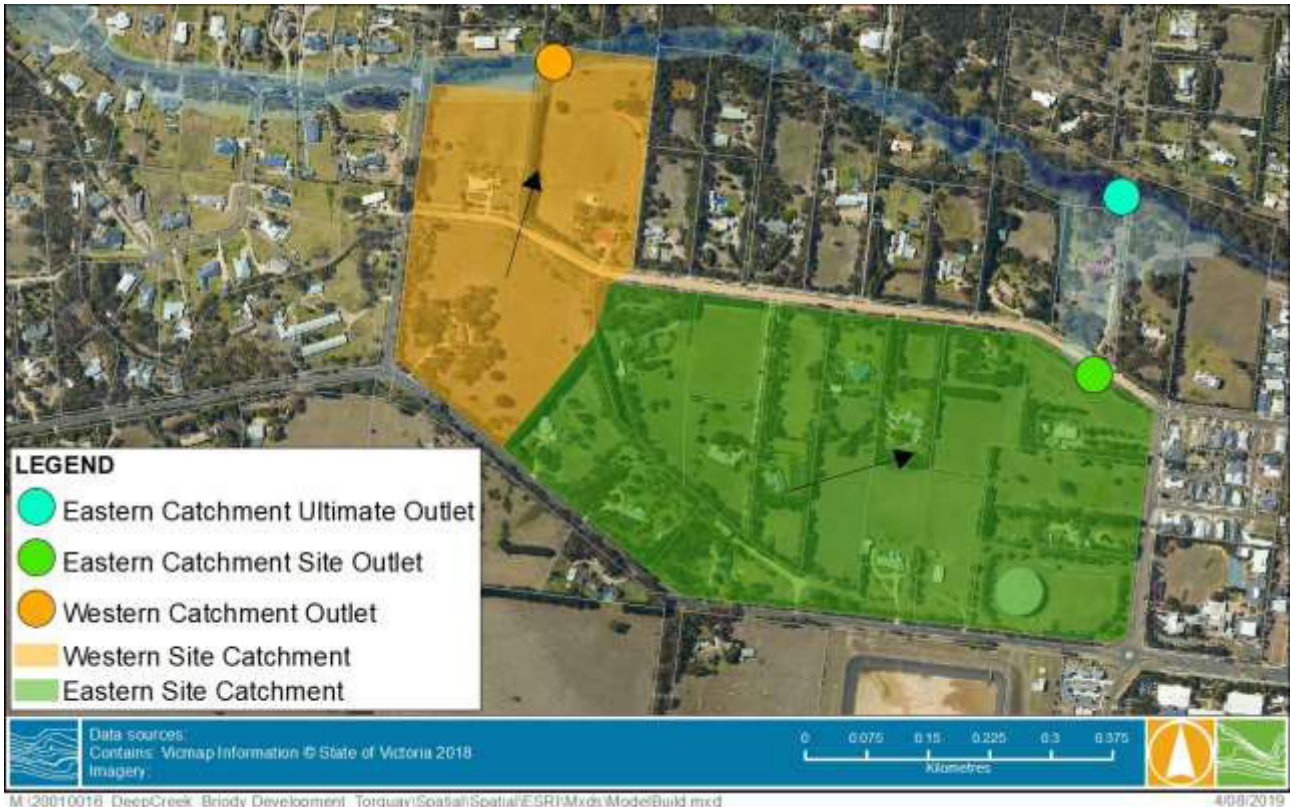
FIGURE 4-3 SITE DRAINAGE CATCHMENTS AND OUTLETS
