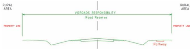
Figure 4 – Demarcation Arrangements for Typical Rural Arterial Roads
