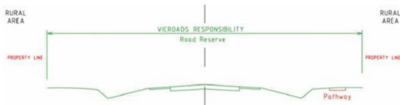
Figure 4 – Demarcation Arrangements for Typical Rural Arterial Roads
