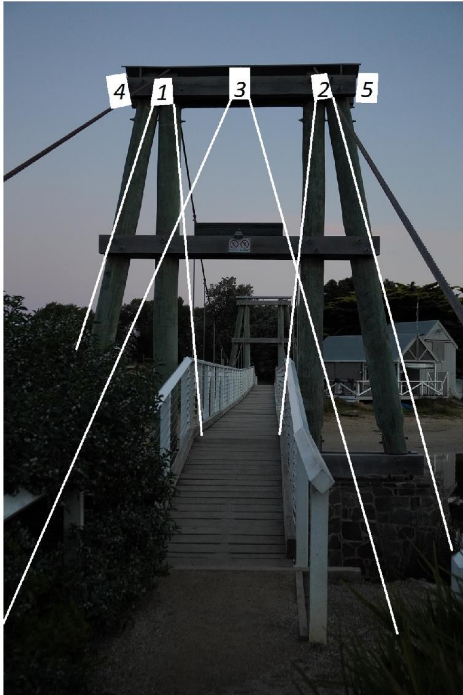
Sketch B) Fixtures 1 & 2 focused on hardwood poles, repeated on other side of tower, not shown. Fixture 3 additional installation to light bridge entrance decking. Fixtures 4 & 5 additional installation to light bridge span proper
