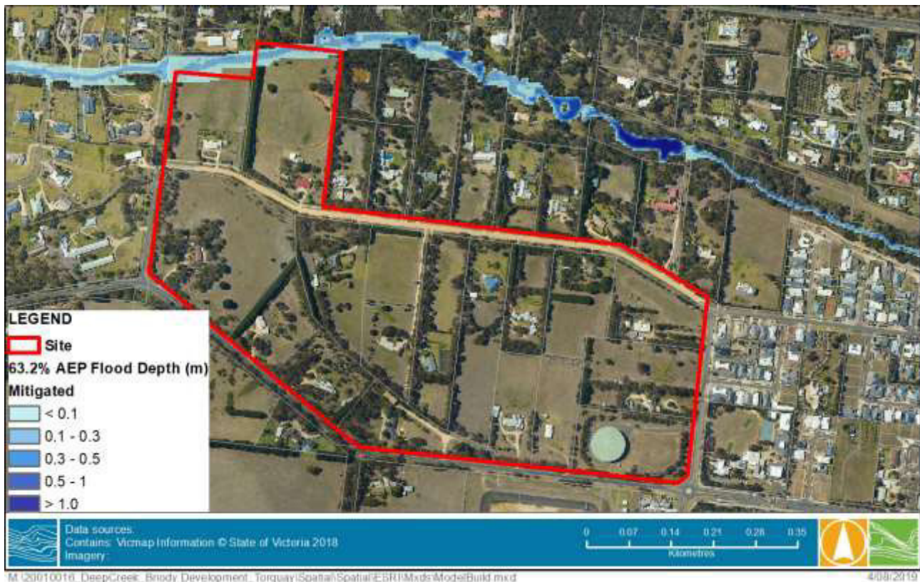
FIGURE 4-9 63.2% AEP FLOOD DEPTH – MITIGATED CONDITIONS
