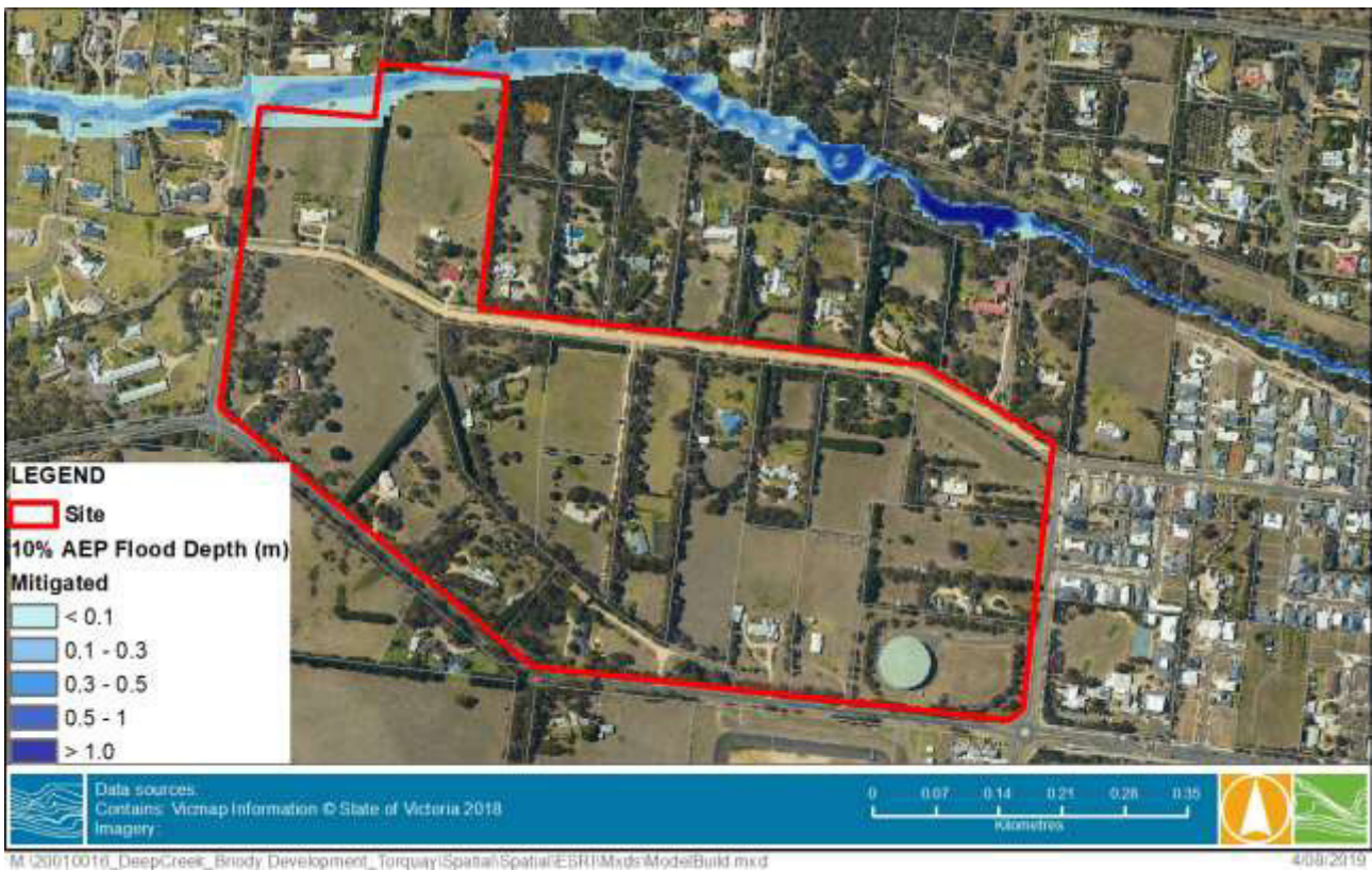
FIGURE 4-8 10% AEP FLOOD DEPTH – MITIGATED CONDITIONS
