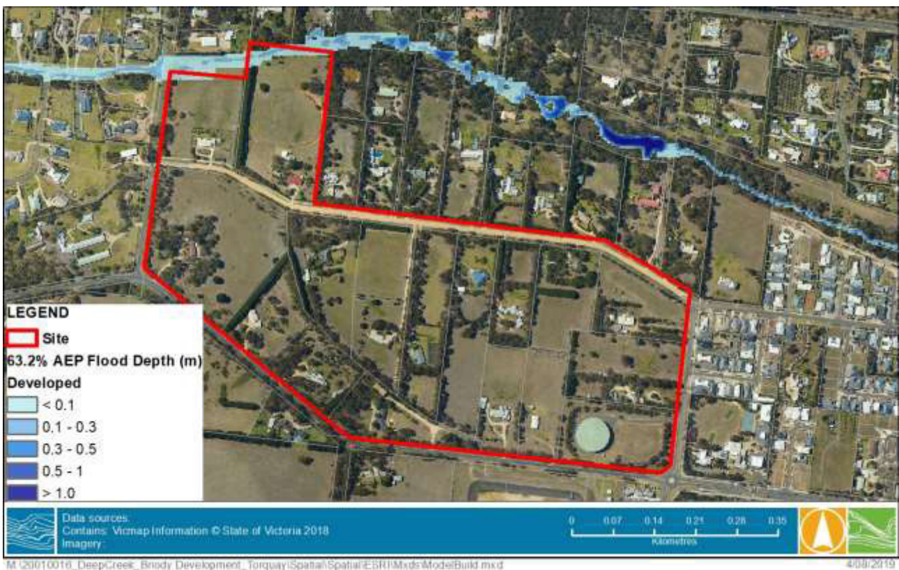
FIGURE 4-6 63.2% AEP FLOOD DEPTH – DEVELOPED CONDITIONS
