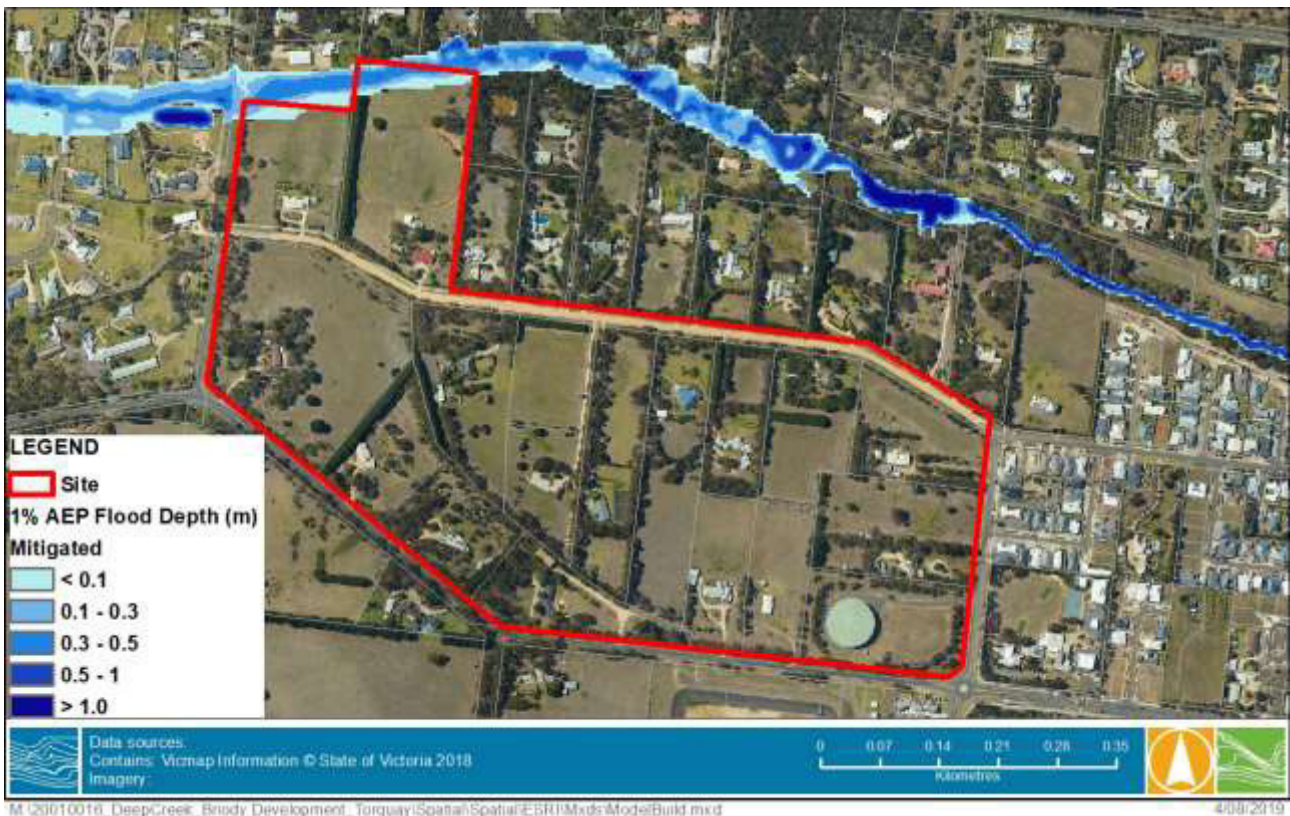
FIGURE 4-7 1% AEP FLOOD DEPTH – MITIGATED CONDITIONS
