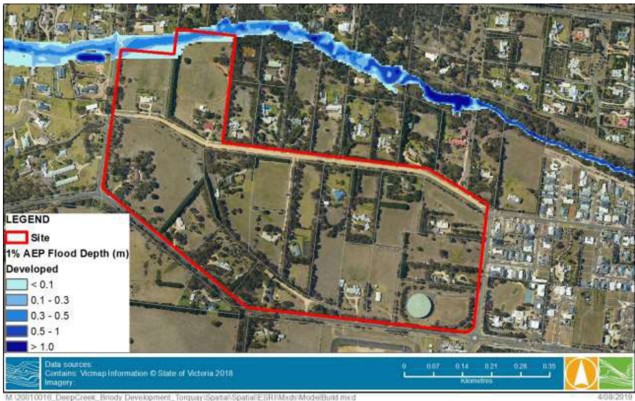
FIGURE 4-4 1% AEP FLOOD DEPTH – DEVELOPED CONDITIONS
