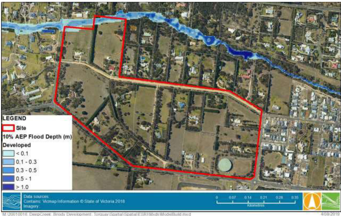
FIGURE 4-5 10% AEP FLOOD DEPTH – DEVELOPED CONDITIONS
