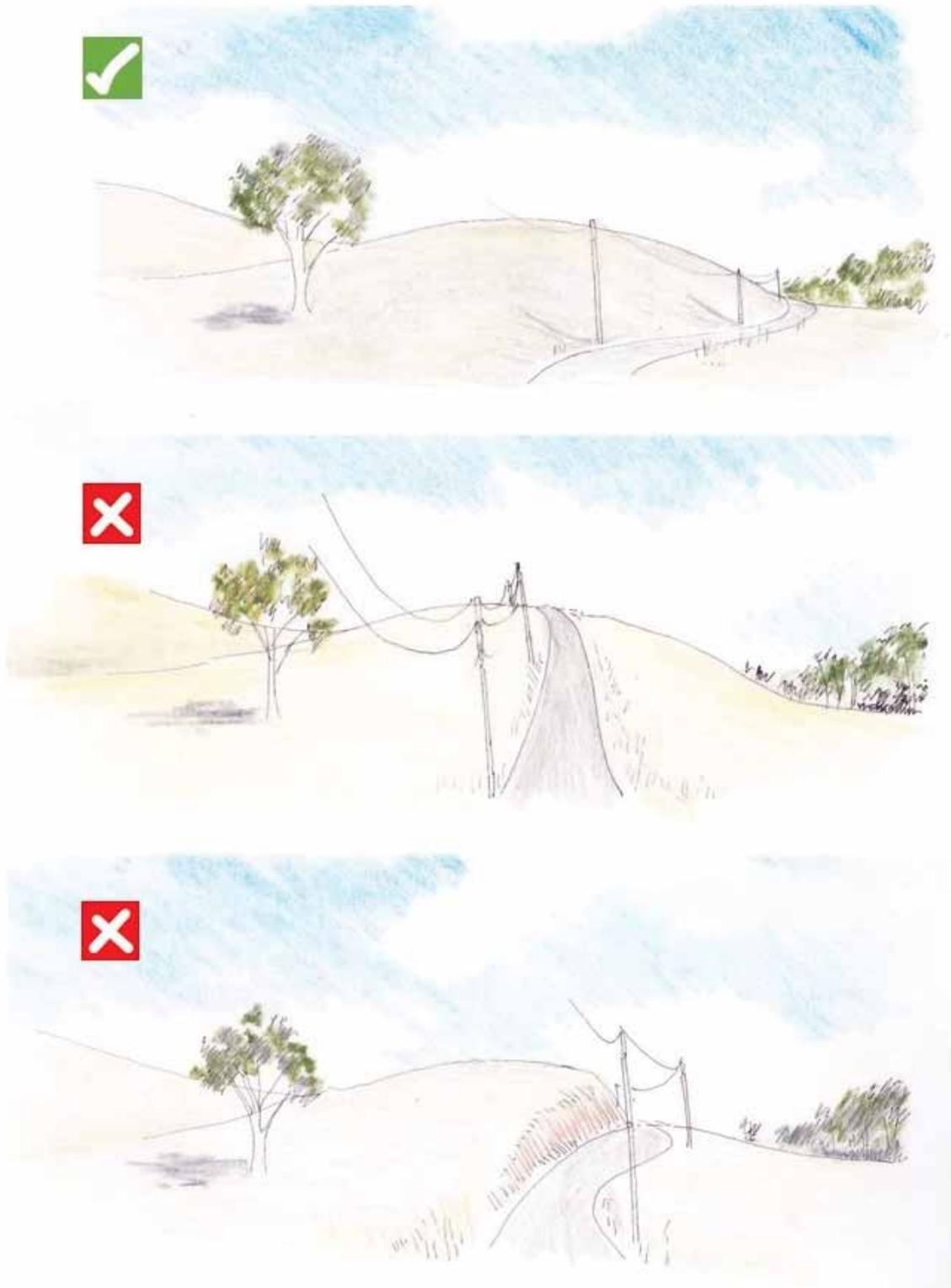
Figure 22: Access design on undulating land
