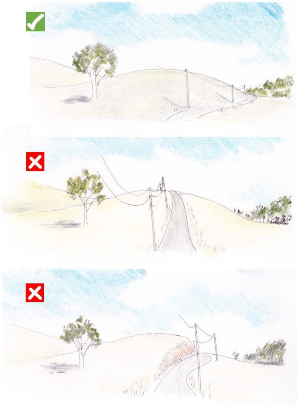
Figure 22: Access design on undulating land
