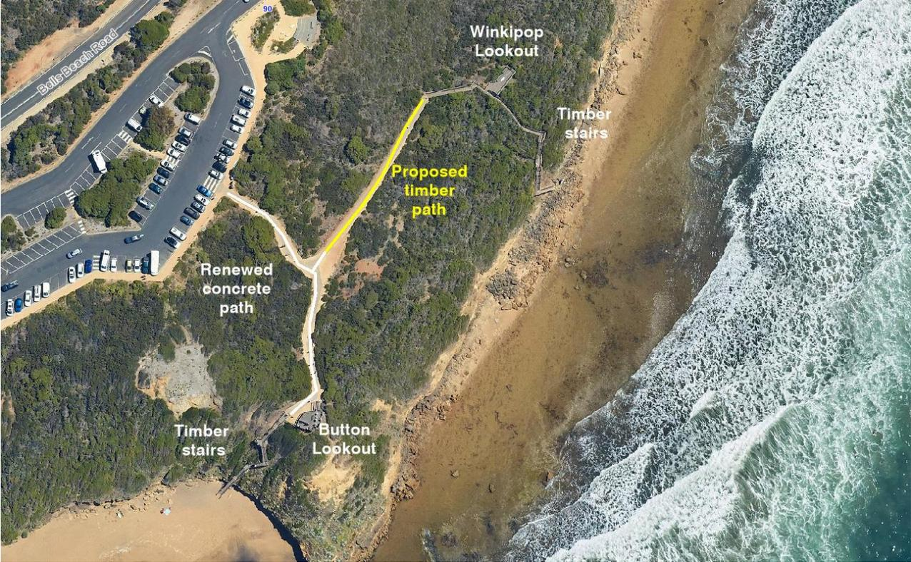
Figure 4 Close up of the site of the proposed elevated timber pathway, replacing concrete
