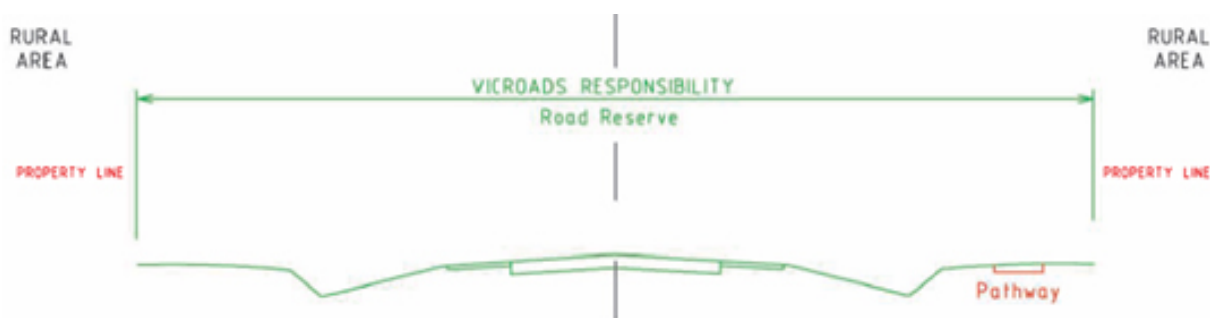
Figure 4 – Demarcation Arrangements for Typical Rural Arterial Roads
