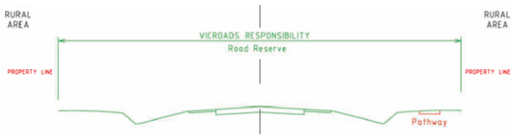
Figure 4 – Demarcation Arrangements for Typical Rural Arterial Roads
