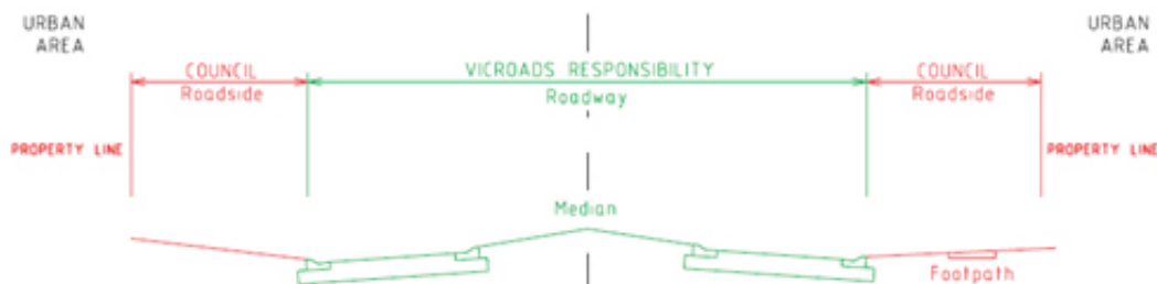
Figure 3 – Demarcation Arrangements Urban Arterial Roads
