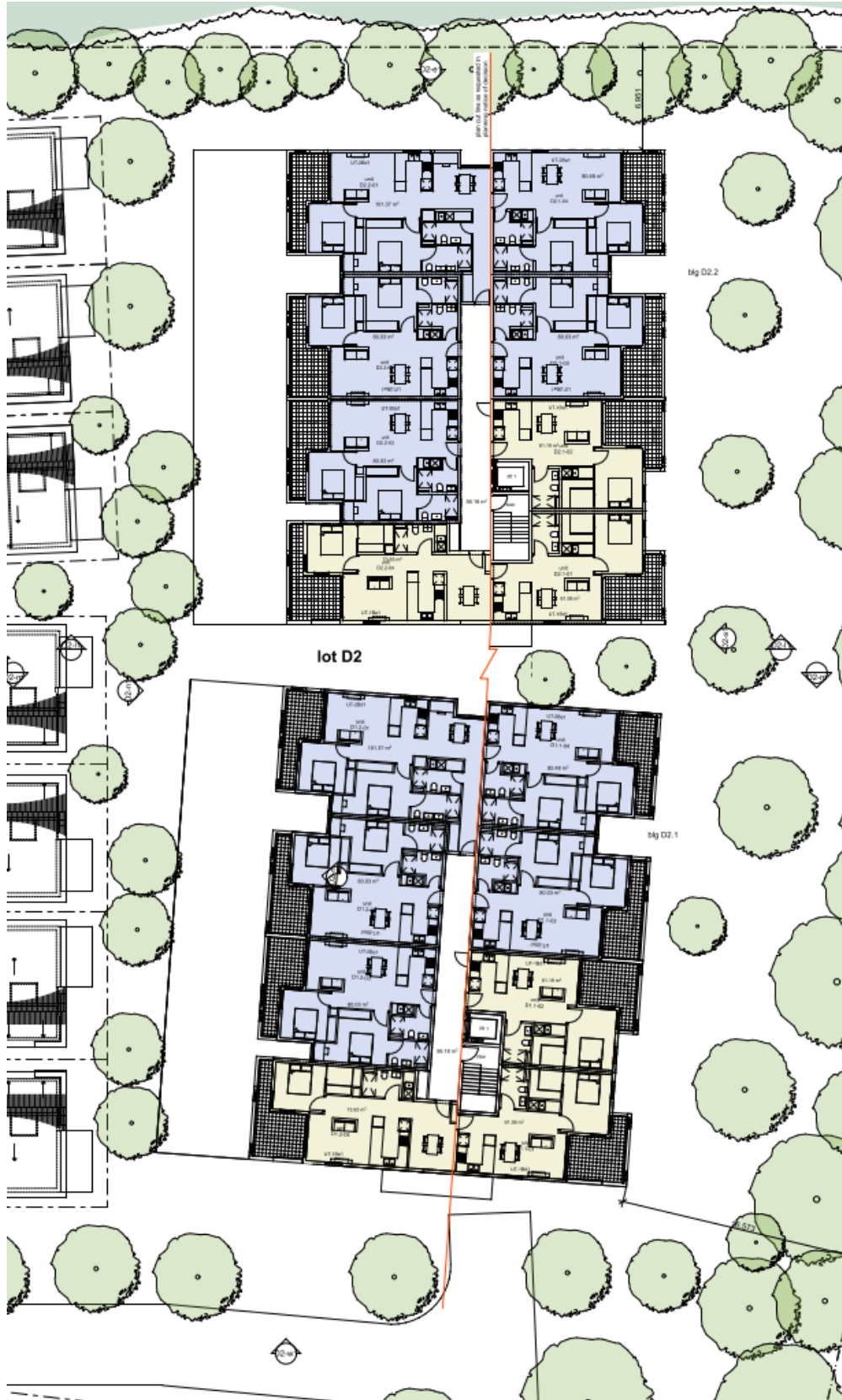
Figure 17 – Lot D1/D2 Apartment Building First Floor Plan
