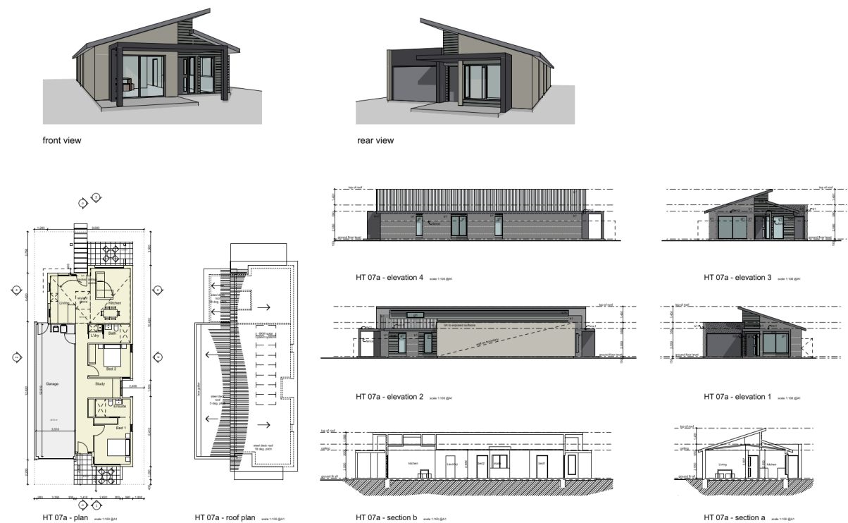
Figure 23 – Unit Type 7A Plans
