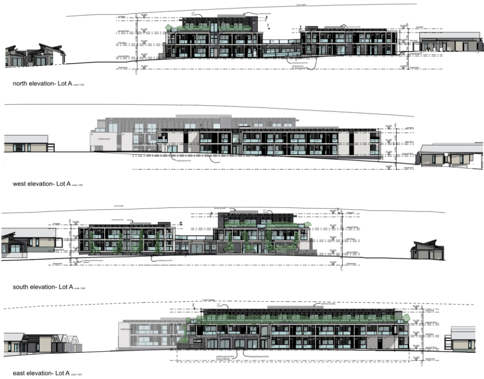
Figure 9 – Lot A Apartment Building Elevations Plan
