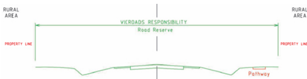
Figure 4 – Demarcation Arrangements for Typical Rural Arterial Roads
