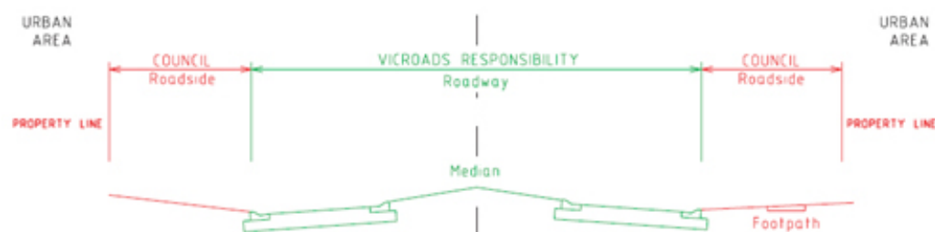
Figure 3a – Demarcation Arrangements Urban Arterial Roads
