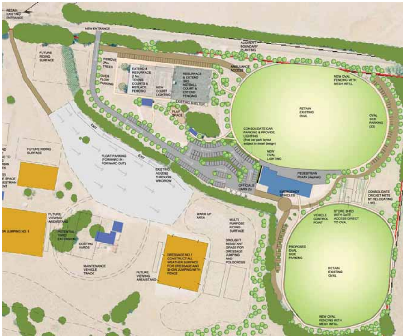
Figure 13 – Extract of Master Plan showing vehicle circulation (refer to Appendix F for full Master Plan)
