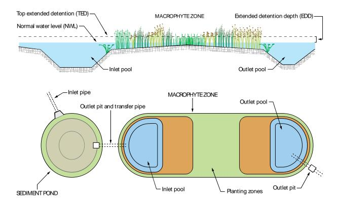
*Figure 2 Typical layout of a constructed treatment wetland.*
