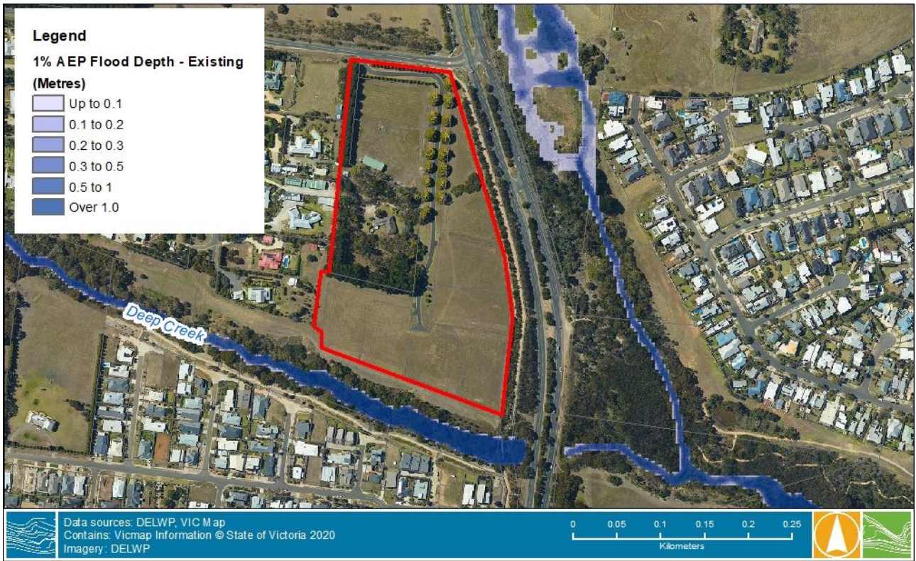
FIGURE 14 DEEP CREEK 1% AEP FLOOD DEPTH
