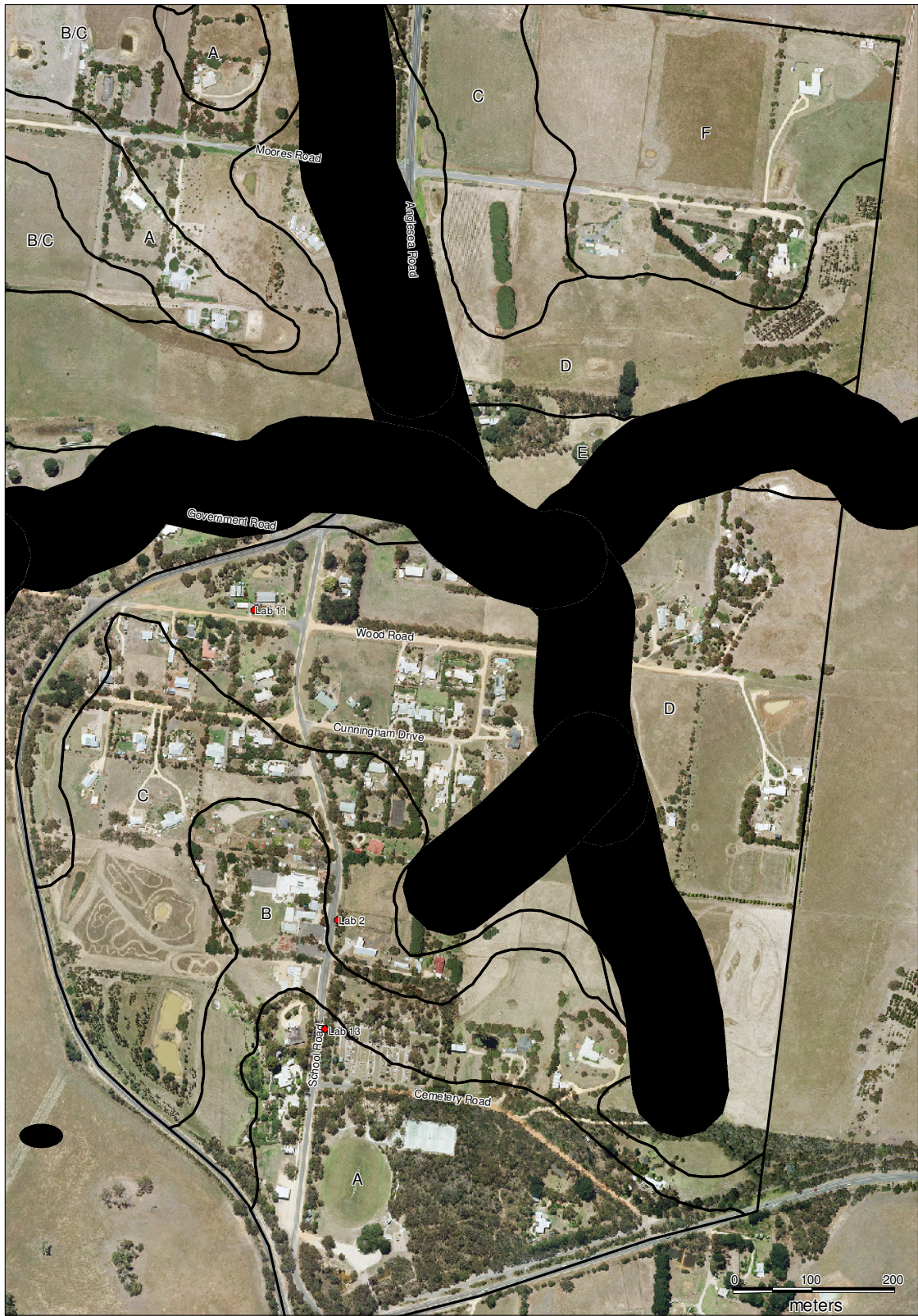
Map 3: Aerial photograph, superimposed with stream setbacks, soil zones (A to F) and sample points for soil sent for lab analysis.
