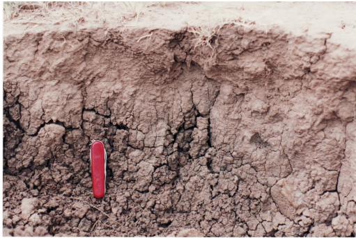
Structureless topsoil over strongly angular blocky structured clay subsoil – macroscopic assessment (scale: pocket knife)
