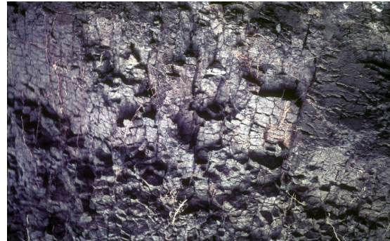
Strongly structured clay subsoil, prismatic and breaking apart in coarse angular blocks – macroscopic assessment
