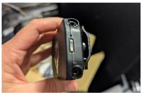
4. Display will come on, will show battery, should always be fully charged. User can change volume with buttons on the front. There is only 1 channel.
