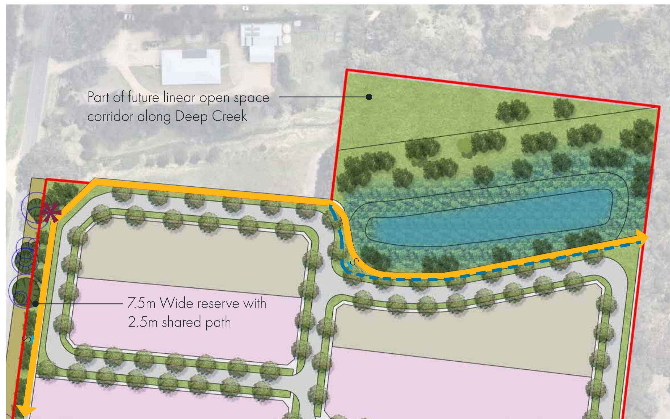
ENLARGEMENT PLAN 01 - DRAINAGE BASIN
