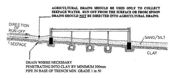
Problems can occur at sloping sites where topsoil, silts, and sands overlay stiff clay. The downhill flow of seepage water can be stopped at a footing which is excavated into the clay. This dammed up water can produce undesirable wet areas. It may prove necessary to provide an agricultural drain to remove this water (see sketch above).
