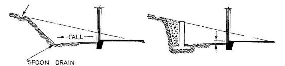
• On slope or low lying sites concrete slabs must be raised off the ground and adequate drainage provided so as to prevent any possibility of storm water inundations.
