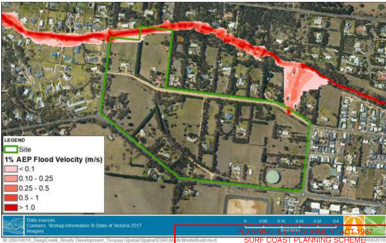
FIGURE 3-5 DEEP CREEK 1% AEP FLOOD VELOCITY
