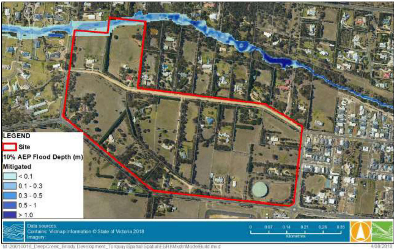
FIGURE 4-8 10% AEP FLOOD DEPTH – MITIGATED CONDITIONS
