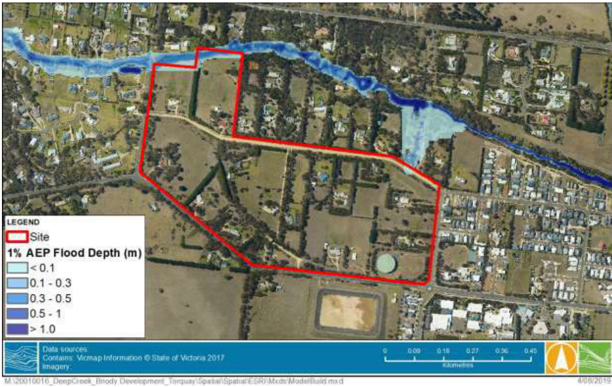
FIGURE 3-4 DEEP CREEK 1% AEP FLOOD DEPTH
