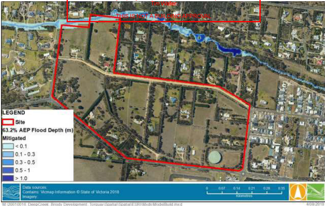
FIGURE 4-9 63.2% AEP FLOOD DEPTH – MITIGATED CONDITIONS
