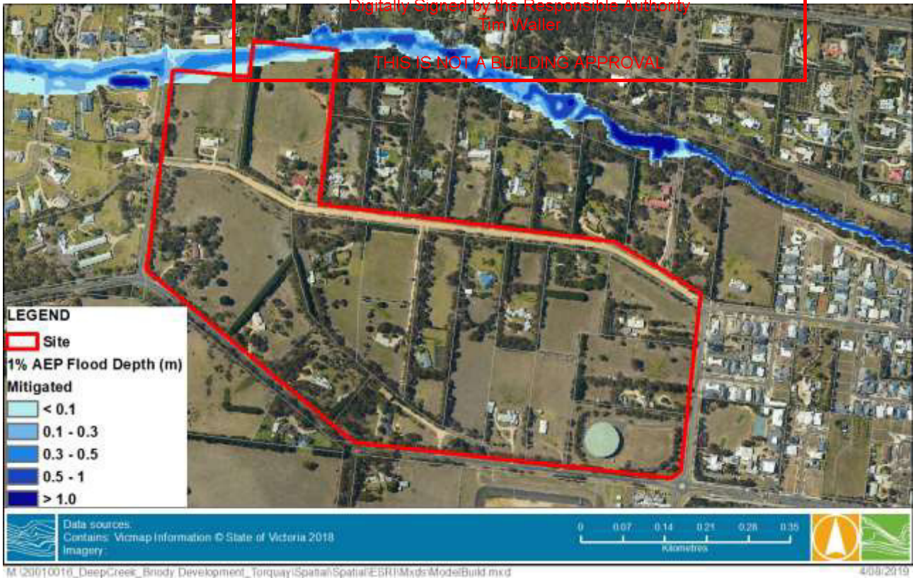
FIGURE 4-7 1% AEP FLOOD DEPTH – MITIGATED CONDITIONS
