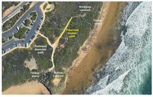
Figure 4 Close up of the site of the proposed elevated timber pathway, replacing concrete
